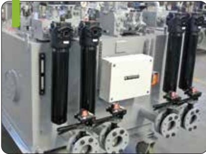
Main engine driven power unit hydraulic tank.
